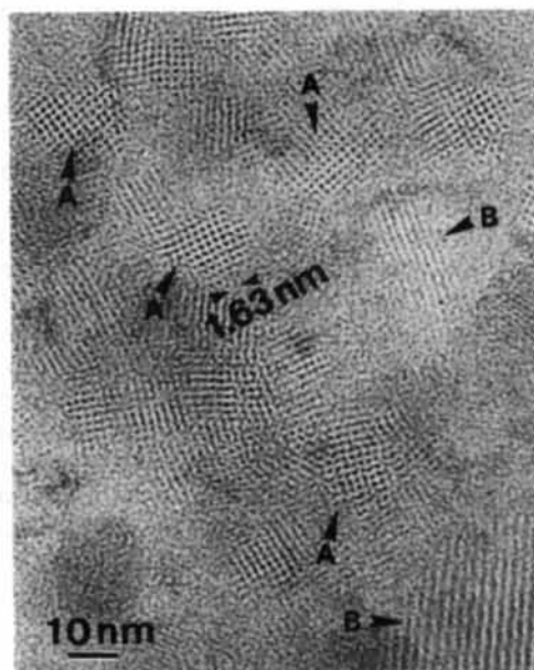
Fig. 9. Electron micrograph of a thin film of the CuPc(CN)_8-Cu complex crystal produced on a Cu film.
